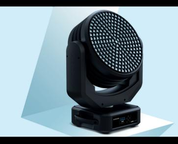
The WILDSUN™K25 features powerful tri-phase stepper motors that allow fast, accurate and silent positioning. Its optical zoom has a 6:1 ratio with a zoom range of 10° to 60°. The precision electronic dimming function can be fine-tuned with significant flexibility. The light output is equipped with a honeycomb filter to prevent glare. The user can control each concentric circle individually to adjust the luminaire's power accordingly.
